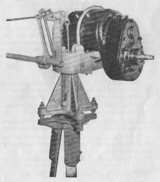
Plants are sent from the factory with the gear boxes filled with suitable oil. This oil is suitable for 4-5 years' running. When replacing or renewing oil, use Shell Retinax Light or similar grade gear oil.
